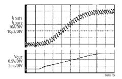
Figure 4. 1.2V, 100A Load Current Step (Top Trace) and Start-Up (Bottom Trace)
